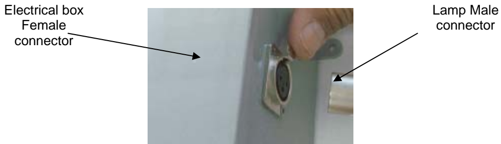
Figure 2. Lamp connector connection with electrical box
